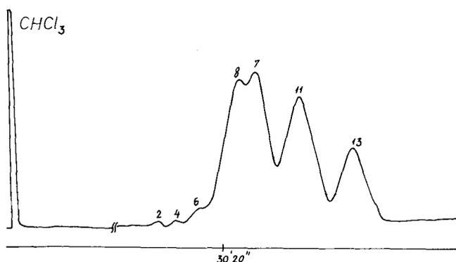
FIG. 1. Gas chromatogram of sterol fraction on 1.5 m OV-17 glass column.
