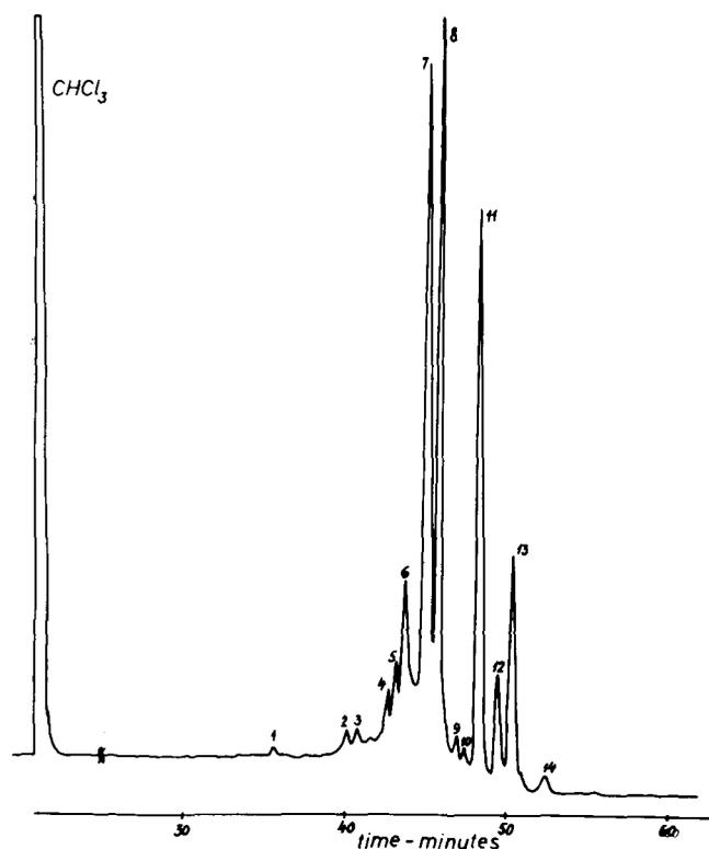
FIG. 2. Gas chromatogram of sterol fraction on 40 m SE 30 glass capillary column.
